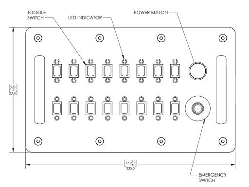
The PRC-16-MK2 16-channel control box has been designed for chain hoist control systems. Its new technology allows connection via an RJ45 connector. Tjami or Veam adapters are available on request.
